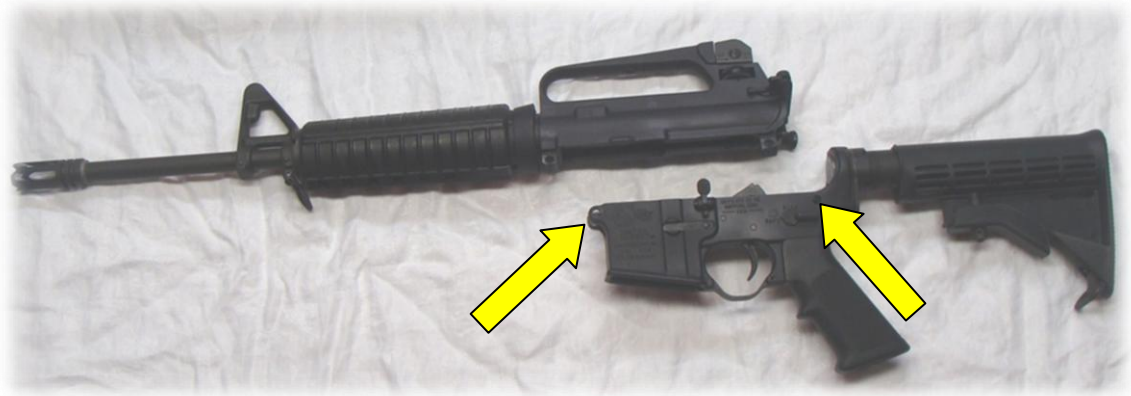
Figure 29: Front and Rear Takedown Pins
